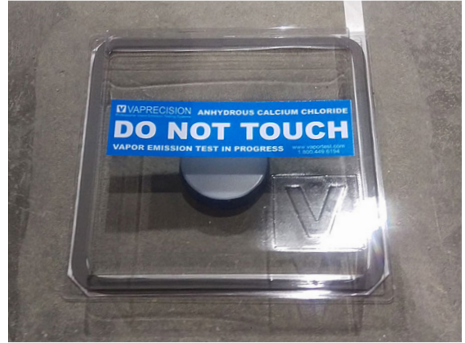
Figure 2.16 – Calcium Chloride Test in place (Photo Courtesy of Vaprecision).
