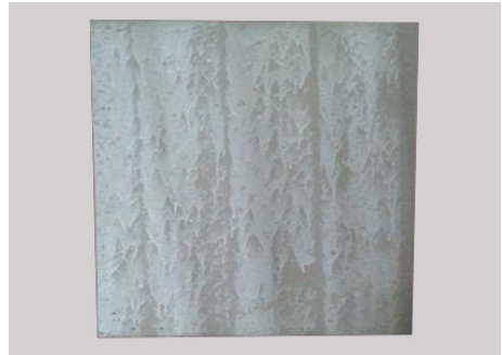
Figure 8.1 — Example of kiln release present on tile back.
