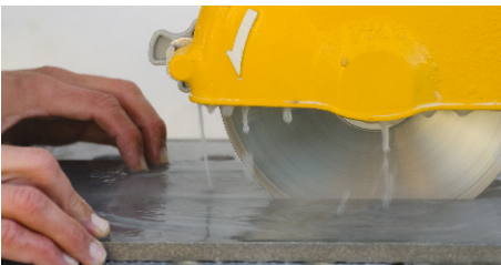
Figure 8.4 — A commercial grade wet saw is ideal for cutting all types of tiles in industrial applications.
