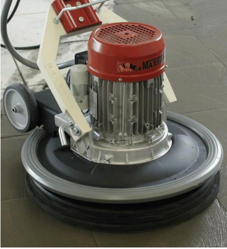
Figure 8.10 – Raimondi USA – Power grouting
