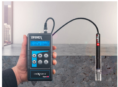
Figure 2.17 – In Situ Moisture Testing.
