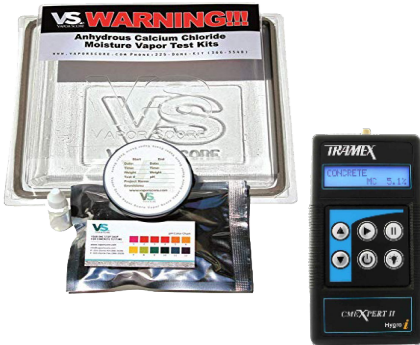
Figure 2.5 – ASTM F1869 Calcium Chloride Test Kit and ASTM F2170 Relative Humidity Meter.
